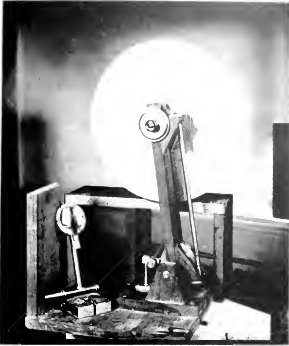
Figure 5.—EXPERIMENTAL GRAPHOPHONE photographed in 1884 at the Volta Laboratory. This is similar to one preserved at the Smithsonian Institution. ( Smithsonian photo 44312 D. )
